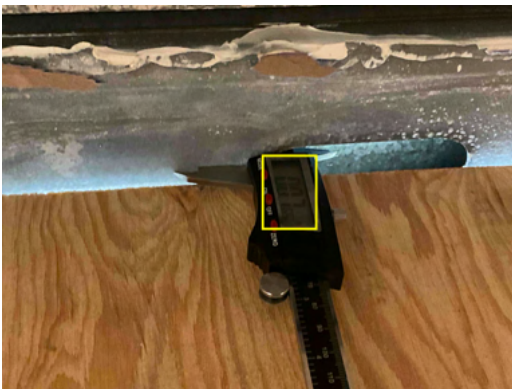
Photo 11 Unit No. 200 - View of existing framing measuring 0.07" which equates to a 14 Gauge metal stud.
