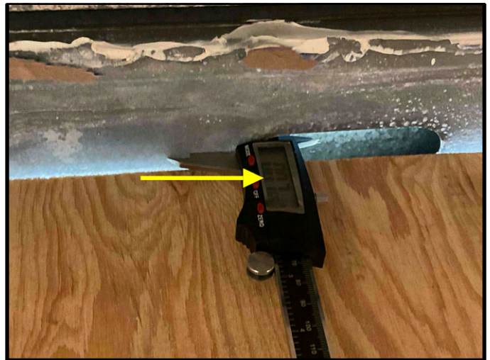
FIGURE 10 - Unit No. 200 - View of existing framing measuring 0.07" which equates to a 14 Gauge metal stud.
